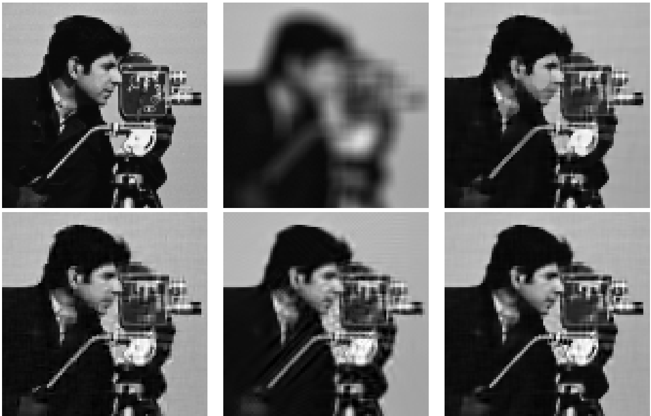
Figure 1. Deblurring of the Cameraman image, scenario 3. From left to right and from top to bottom are presented zoomed fragments of the following images: original, blurred noisy, reconstructed by CGMK [6] (ISNR 9.15), L0-AbS [7] (ISNR 9.10), DEB-BM3D [8] (ISNR 8.34) and by proposed IDD-BM3D method (ISNR 10.45).
